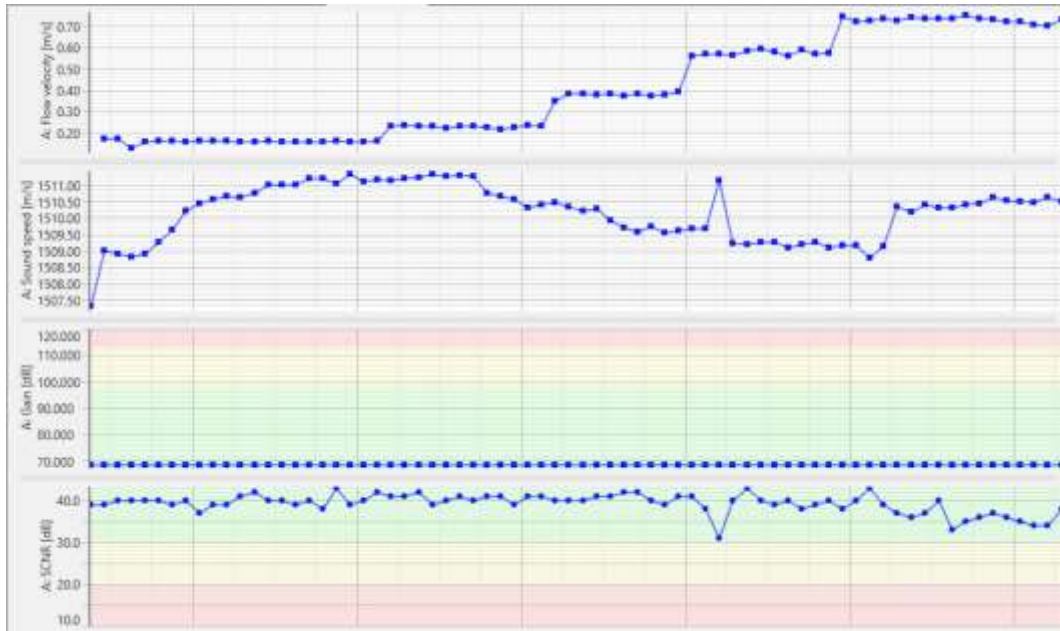
Fig. 6. Transitional low flow to high flow profile
