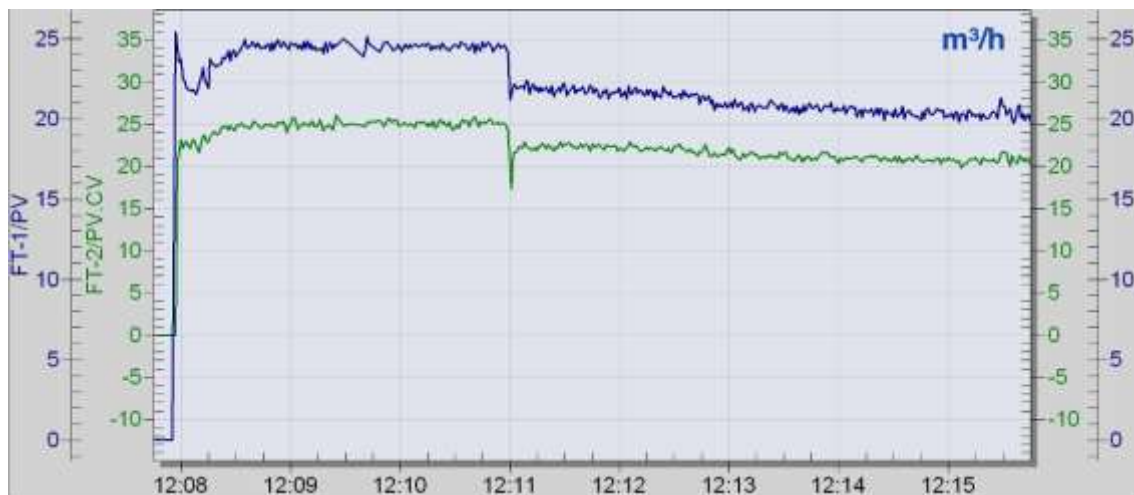
Fig. 7. Comparison of flow profile of tested device against reference flowmeter
