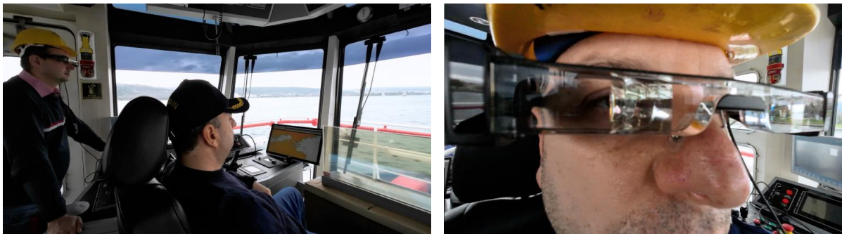
Fig. 11. Maneuver execution using the Pilot system and AR headset during daylight for validation of positional accuracy and real-time dynamic performance
